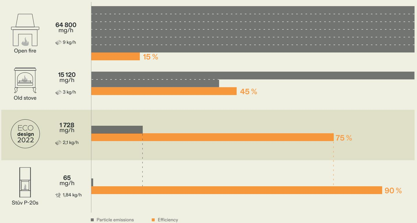
With its high level of efficiency and incredibly low fine particle emissions, the Stův P-20s performs better than the Ecodesign 2022 standard.
